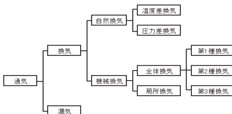
Fig. 1 Types of ventilation (ventilation and leakage) 9)
